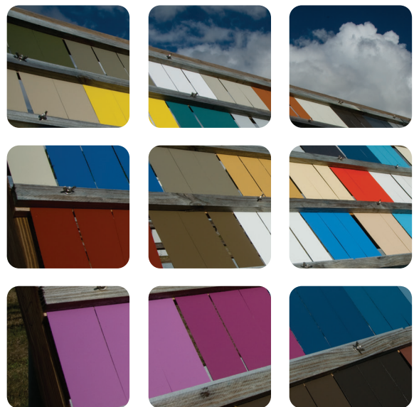
Valspar's 70% PVDF Fluoropon® Coating versus Competitor A: Gallery Blue Natural Weather Exposure, Ft. Myers, FL, 9+ Years Exposure
