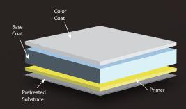
Extrusion is a three-coat PVDF resin system with a total Dry Film Thickness (DFT) of 2.2 - 3.0 mils.
